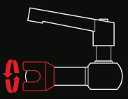
Cuffs can rotate independently of arms and provide additional positioning options and notch locations.
