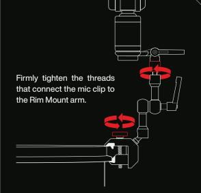
Firmly tighten the thumb screw. Often times an extra turn or two is necessary as the Rim Mount teeth compress against the rim of the drum.
